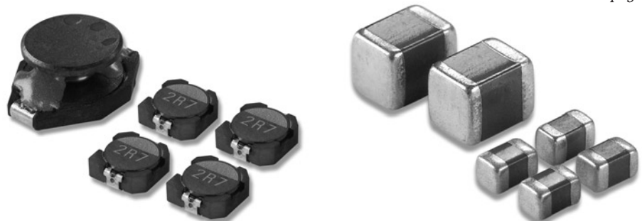
Figure 1. How does a multiphase boost converter improve on its single phase counterpart? First of all, a multiphase topology saves space and simplifies layout by removing bulky, hard-to-place components and replacing them with easier-to-fit, low profile components. Inductor and output capacitor size comparison of single-phase and 4-phase circuits.
